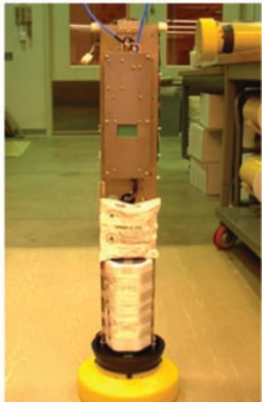
**Drifter with Iridium unit installed**
